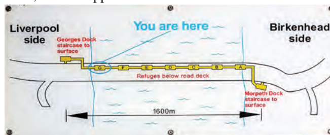
Modern safety signage showing the new refuge rooms, built deep in the tunnel after the Mont Blanc disaster.
